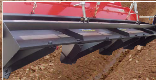
Detalle de conformador Tôle de buttage Ridge former
