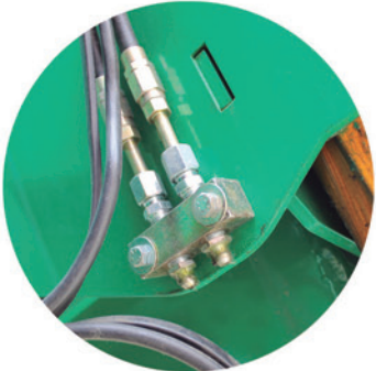
ENGRASE CENTRALIZADO / CENTRALIZED GREASING
