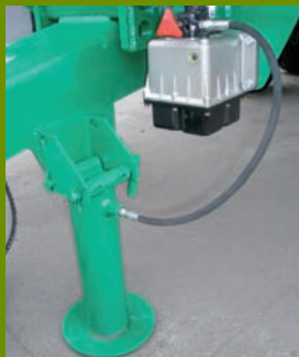
Apoyo hid. y Bomba manual Hydraulic foot and manual pump
