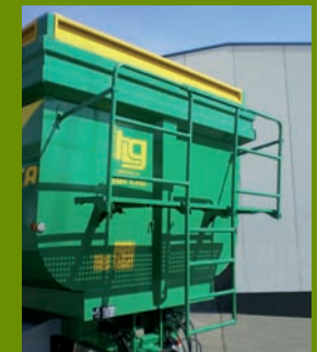
Balconcillo Front small balcony
